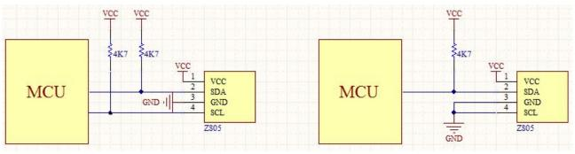
IIC typical application circuit
